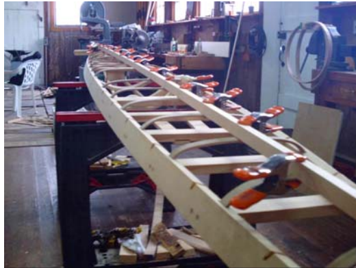
Figure 5. Working out the positioning of the keel before drilling
