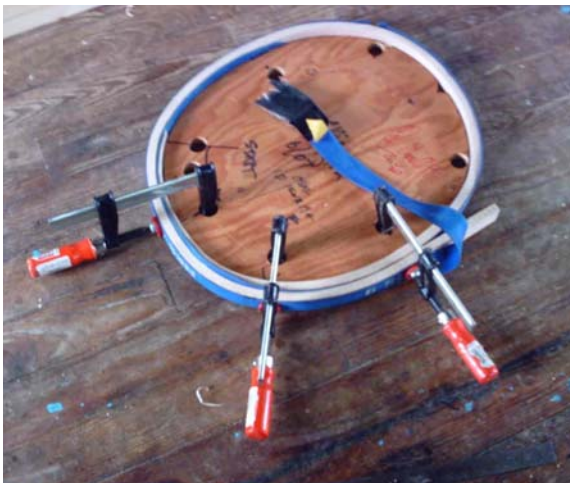
Figure 10. Bending wood around a cockpit template to form a coaming
