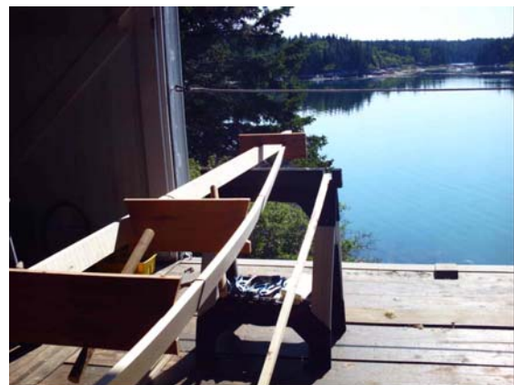
Figure 4. Shaping the gunwales using windlasses to hold their position
