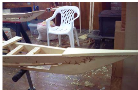
Figure 7. Stabilising the frame to work on a stem piece
